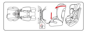
Seat assembly: Lay the seat flat as shown. Hook the backrest into the base and pull it forward until it is secured in an upright position. Secure the buckle on the 5-point safety harness, do this by combining the two buckle pieces together. Insert the buckle ends into the 5-point harness buckle.
