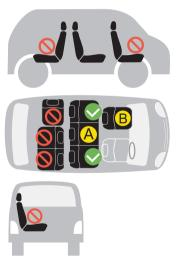
The suitable location for installation in the car is shown on the left:
